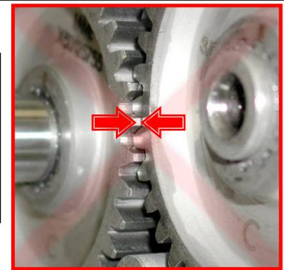
5- BEFORE APPLYING THE SEEGER, CHECK THE POSITION OF ALL GEARS AND THAT ALL REFERENCE MARKINGS ARE ALIGNED CORRECTLY.
